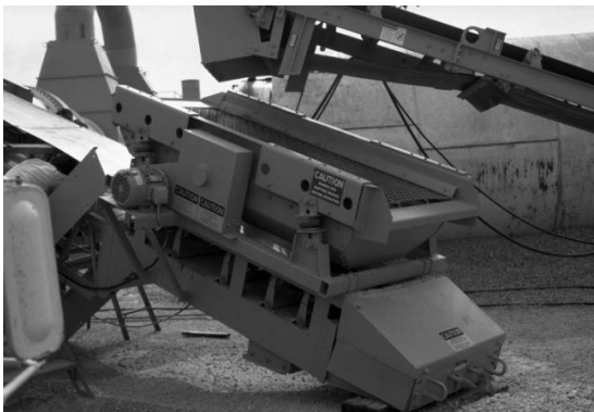
Dryer-Drum Cold Elevator Scalping Screen
