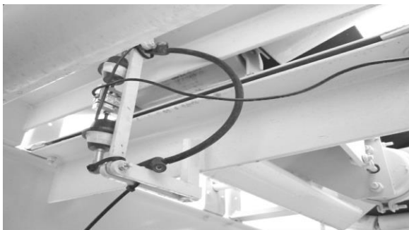
Weigh Bridge Load Cell
