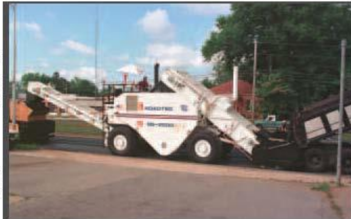
SHUTTLE BUGGY MATERIAL TRANSFER VEHICLE F-38
