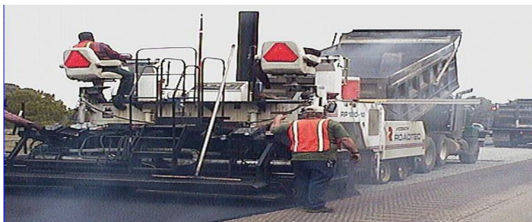
New Modern Electronically Controlled Paver
