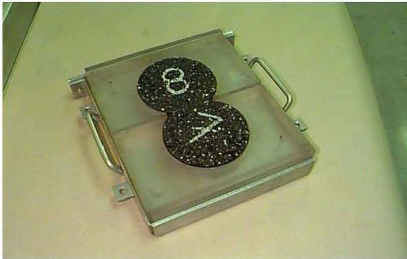
Figure 1 —Cylindrical Specimen Mounting System
