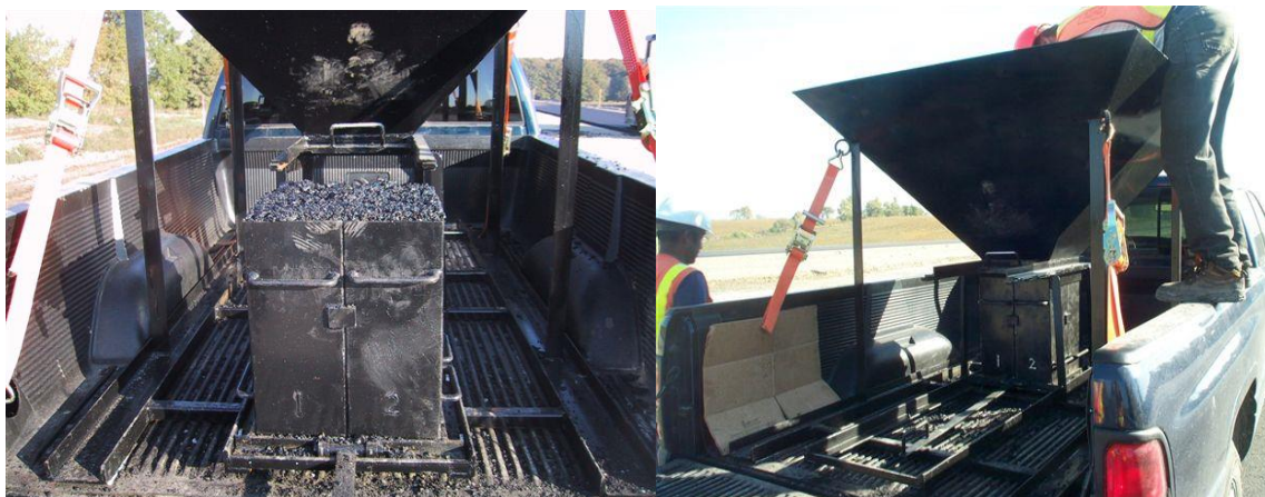
Figure 4. Additional Examples of MTD Sampling Devices
